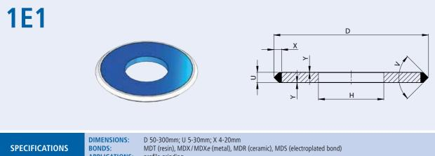
APPLICATIONS: profile grinding CONCENTRATION SHAPE D BOND GRIT U X V H Y SAMPLE ORDER 1E1 300 20 15 90 127 0,2 MDT D126 C85
